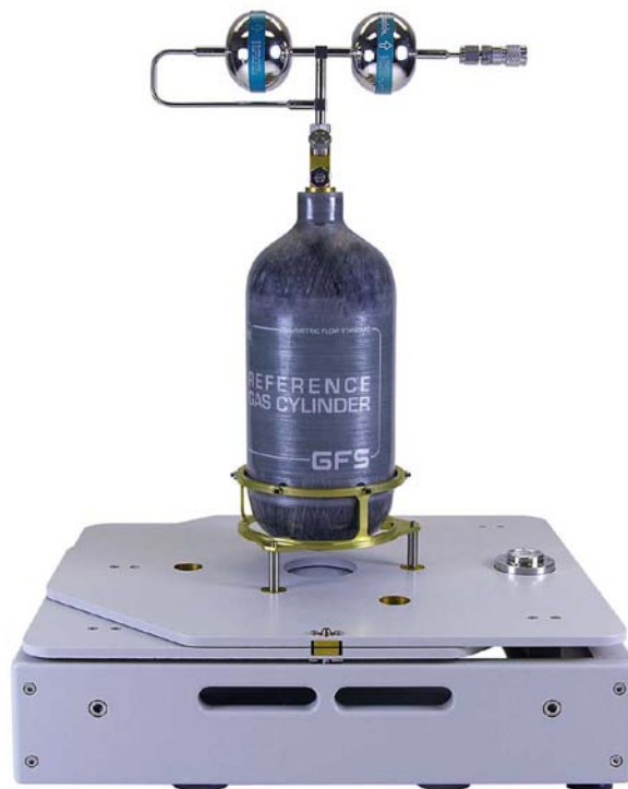
Figure 2. Reference gas cylinder resting on GFS balance and AMH-GFS2102
