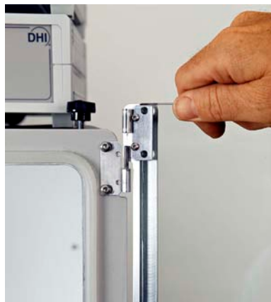
Figure 13. Installation of draft enclosure doors.
