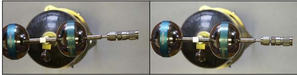
Figure 17. Regulator assembly position before and after tightening for right side operation
