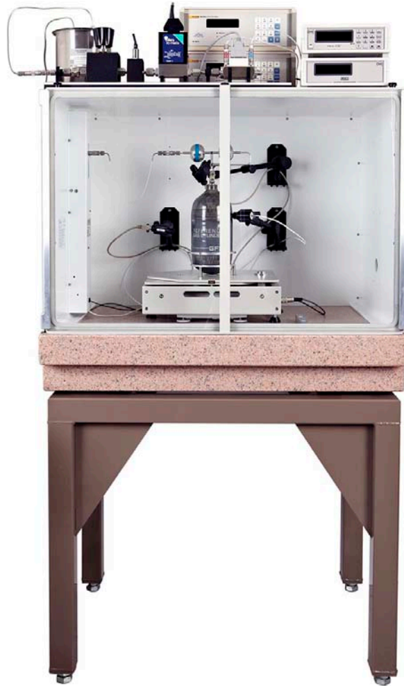
Figure 9. GFS draft enclosure on vibration isolation table
